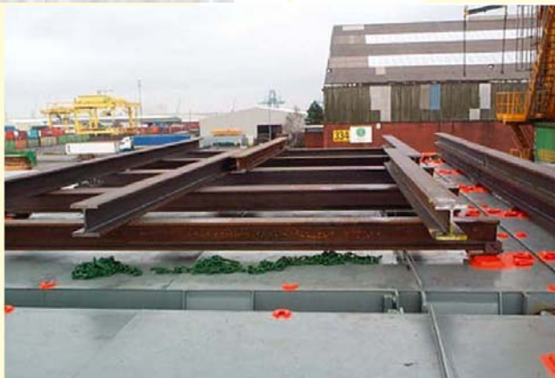
Figure 2.2.9: H-beam bedding system of "Rickmers Hamburg-Class"
